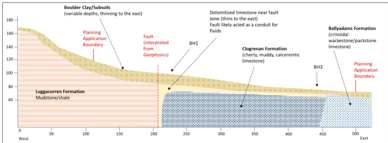
Figure 6-4: Schematic Geological Cross-Section based on SI data
